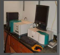
The instrument will excite the molecules of color and measure their wavelengths, which we will see on a graph (spectrum).
